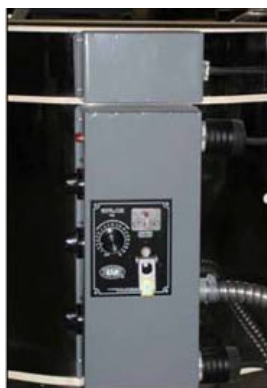
Detach screws from kiln sitter plate
